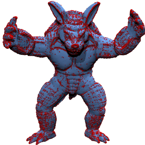
Fig. 13 A mesh of 345,944 faces sampled using 30,392 feature sensitive samples.
