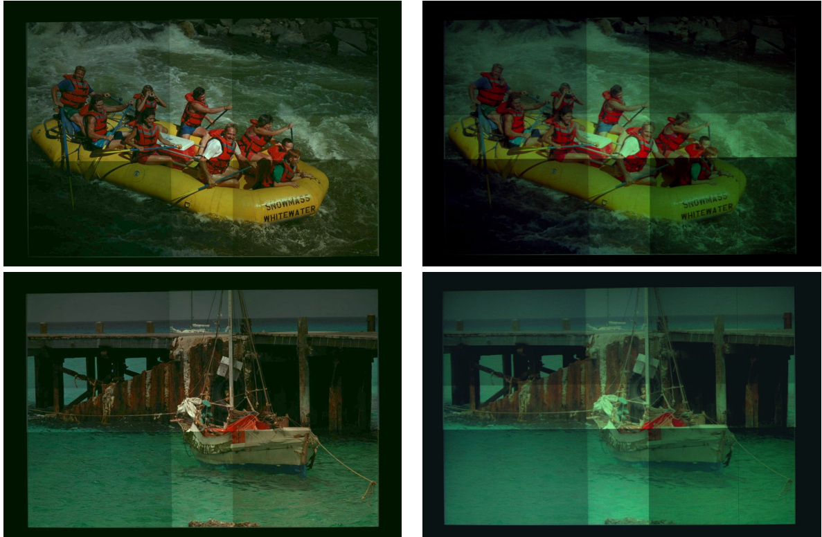
Figure 7: A 2 \times 2 array of four projectors. Left Column: Predicted response generated using our color variation model. Right Column: Actual response generated from a digital photograph.
