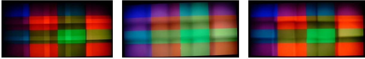
Figure 5: Fifteen projector tiled display at Argonne National Laboratory: before blending (left), after software blending (middle), and after optical blending using physical mask (right).
