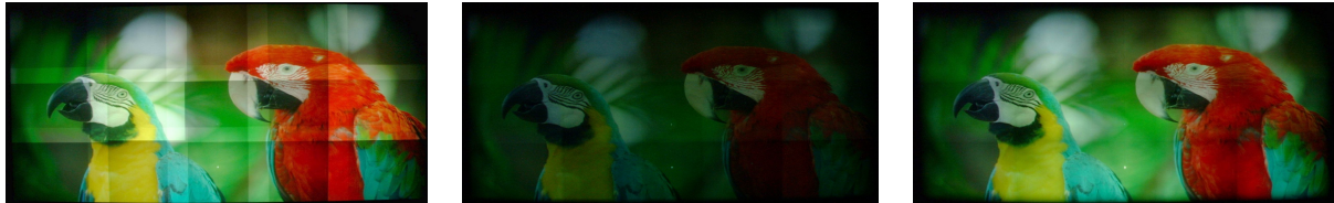
Figure 6: Digital photograph of a 5 \times 3 array of 15 projectors. Left: Before correction. Middle: After intensity matching. Right: After intensity smoothing.
