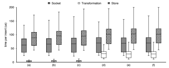
Fig. 4. Time per insert without calling a transformation function (a–c), and with calling a transformation function to convert the representation (d–f).
