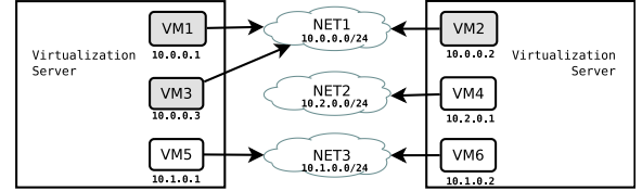
Fig. 5: Virtual network topologies used to evaluate MAC address resolution. All logical networks were implemented over the physical network in Fig. 3.
