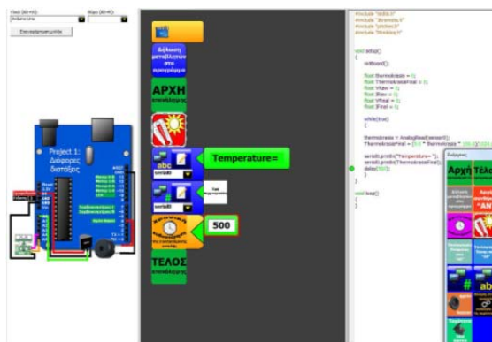
Figure 6: Definition of new experiments using Minibloq visual programming language. The teacher selects predefined experiment blocks (from toolbar at bottom right) and drags them to the central panel. Possible configurations can be made by clicking graphical objects. Concurrently the corresponding Arduino code is presented at right panel while at the left panel a hardware view of Arduino connections is depicted.
