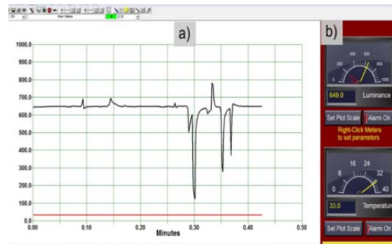
Figure 5: Real time presentation of acquired values that sent over USB in real time using Stampplot software: a) Data from channel 1 and b) data from channel 1 (top gauge) and channel 2 (bottom gauge).
