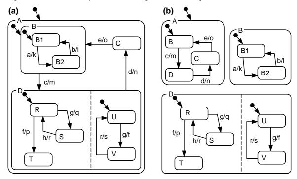
**Explanation of symbols.** States and statecharts are denoted by rectangles, transitions by arrows. x/y denotes a triggering event x and a triggered action y for a state transition. Arrows originating in a black dot denote initial states on the corresponding nesting levels. A dotted line separates concurrent statecharts. Notations (a) and (b) are equivalent.
