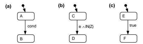
Figure 3. Special kinds of state transitions (the semantics is given below in the text)
