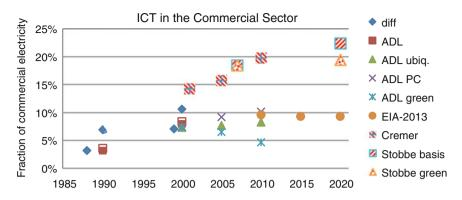
**Fig. 4** Fraction of ICT electricity in the commercial sectors in the US and Germany. Data from different sources: *Data for the US* "diff" = [33, 82–84], all cited from [77, Figs. 2, 3, 4, 5]; "ADL" = [85]; "ADL ubiq", "ADL PC", and "ADL green" = [77, Figs. 2, 3]; "EIA\_2013" = [79]. *Data for Germany* "Cremer" = [80]; "Stobbe basis" and "Stobbe green" = [81]
