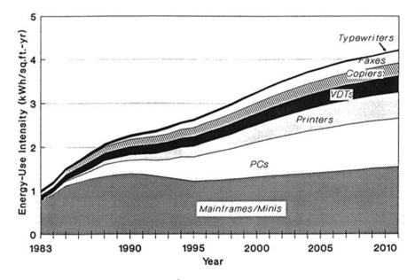
Fig. 3 Energy-use intensity (in kWh/ft<sup>2</sup>  $\times$  year) of office equipment in US office buildings 1983–2010. (*Source* [35, Fig. 7, p. 44], reprinted with permission of Lawrence Berkley National Laboratory)
