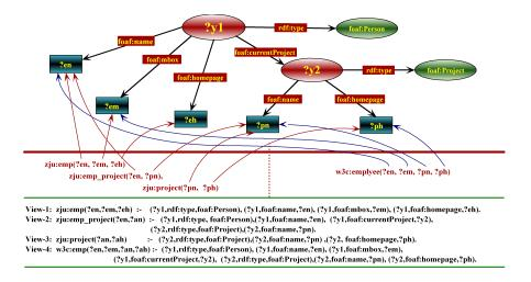
Fig. 3. Mappings from two relational databases with different structures to an ontology. "?en,?en,?eh,?pn,?ph" are variables and represent "employee name", "employee email", "employee homepage", "project name", "project homepage", respectively.
