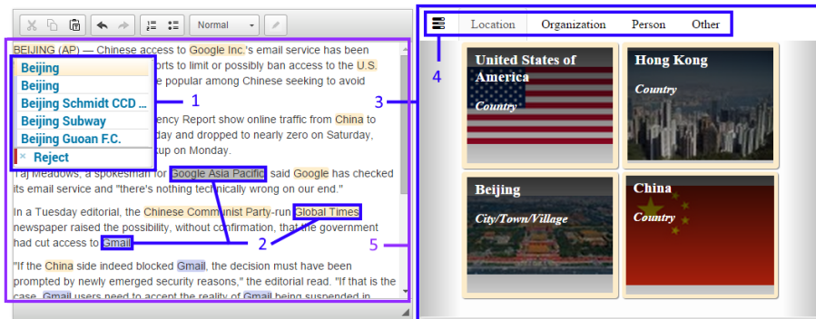
Fig. 3: Main parts of Seed 's front-end: 1- Dropdown menu for viewing, selecting or rejecting an annotation, 2- Suggested as well as confirmed inline annotations, 3- Entity side pane for viewing more information about entities in the text, 4- Controls for Faceted viewing/browsing, 5- Text composition area
