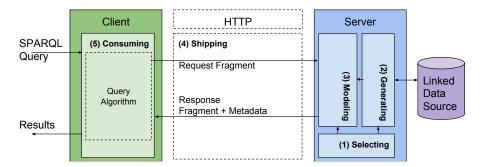
Fig. 1: Complete setup with 5 sequential steps that are subject to research.
