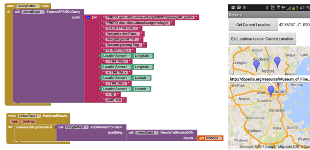
Fig. 1: Consuming Linked Data. Left: Logic used for obtaining the user’s location, constructing a SPARQL query, querying a remote endpoint, and displaying the retrieved results on a map. Right: Output as seen on the phone. ‘QueryButton’ in the blocks editor is the name of the button with the label ‘Get Landmarks near Current Location’ as seen on the phone.
