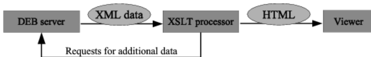
Figure 2: XSLT processor running queries nested in the XSLT script
