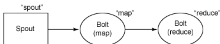
Figure 2. Simple Storm topology for the MapReduce function
