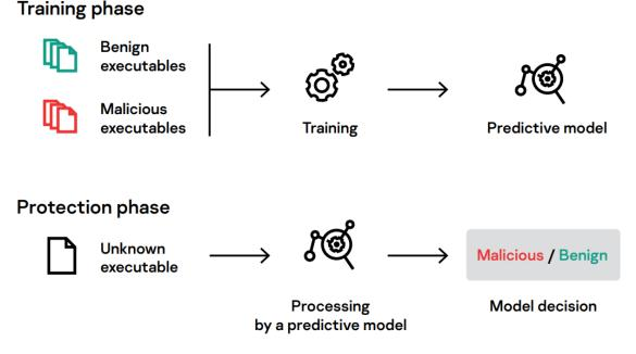
Figure 2.4: Malware detection algorithm life cycle (supervised learning) [36]
