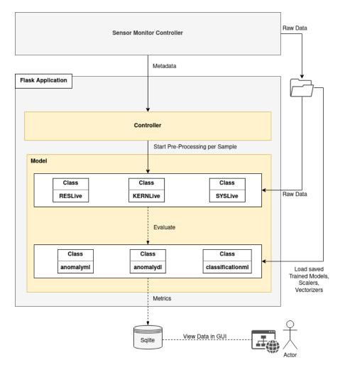
Figure 6.4: Interaction between service classes during live evaluation
