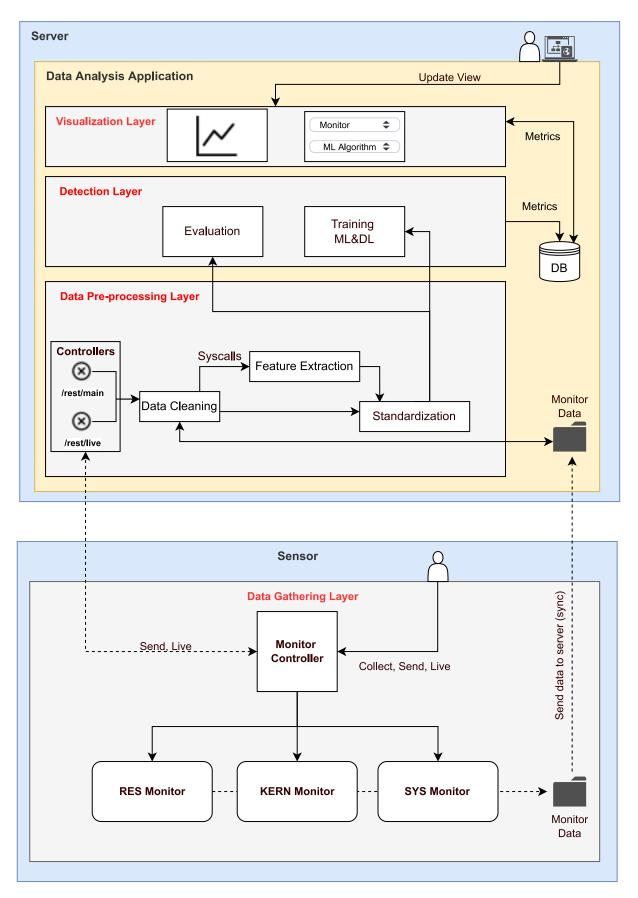
Figure 5.1: Design Overview of the Framework
