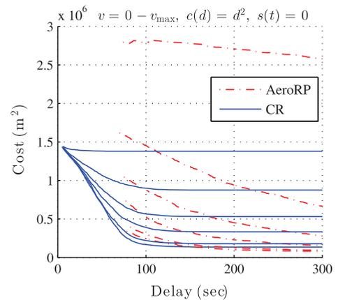
Fig. 3. AC/DC averages in the Uniform Setting for the AeroRP and CR protocols when the nodes have an imperfect knowledge of the future trajectory. The averages plotted are for  $p = 0, 0.02, 0.08, 0.16, 0.32, 1$ . The cost decreases as  $p$  increases.
