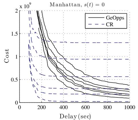
Fig. 5. AC/DC averages for the GeOpps and CR protocols when the nodes only know their trajectories during the time interval  $[t_0, t_0 + T_e]$ , where  $t_0$  is the present time. The averages plotted are for  $T_e = 3, 6, 12, 25, 50$ , and  $\infty$  seconds. The curves are decreasing as  $T$  increases.
