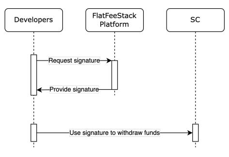
Figure 3.3: Signature mechanism
