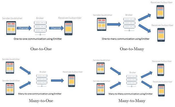
Figure 2.6: Possible Emitter Communication Configurations [22]
