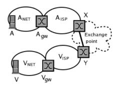
Figure 3.3: Recorded route  $\{A_{gw} X Y V_{gw}\}$  between the hosts A and V. In this example  $A_{gw}$  is the attacker's gateway, *i.e.*, it is the router closest to the attacker A, and V is the victim [6]
