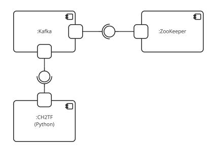
Figure 5.1: The component diagram of CH<sup>2</sup>TF
