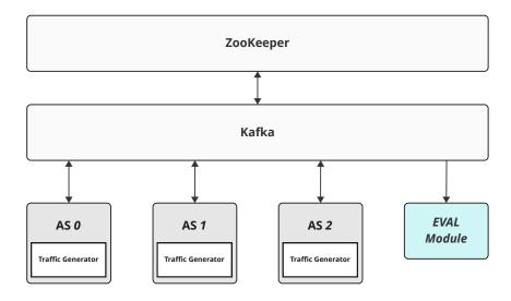
Figure 6.2: Schema of the evaluation architecture used for the attack scenarios. The evaluation module has been added here as an additional Kafka consumer. Also, every AS includes a Traffic Generator that reads the prepared PCAP files to simulate traffic.
