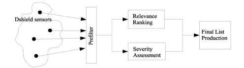
Figure 3.4: Architecture of the blocklisting system [97]
