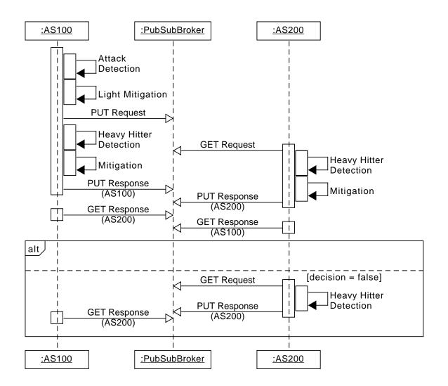
Figure 4.4: Sequence Diagram of  $CH^2TF$ 's communication protocol. In this example, two ASes are used. No HH were found in the alternative path, and AS200 responds accordingly.
