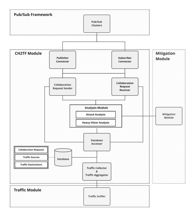
Figure 4.1: Architecture of CH<sup>2</sup>TF. While the *Traffic Module* and *Mitigation Module* are displayed here, they are not part of the project's scope.
