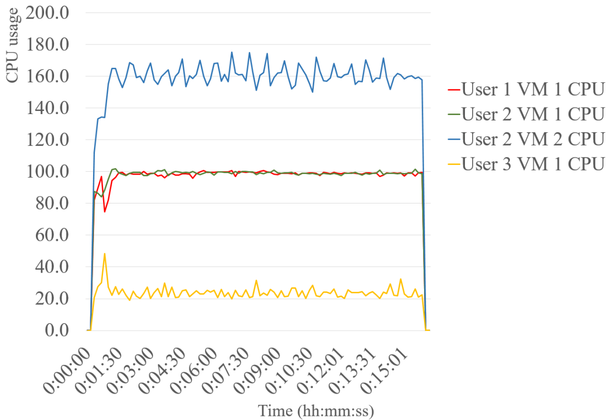
Figure 7.1: Default OpenStack CPU allocation, multinode setup: The VM of User 1 and VM 1 of User 2 belong to node 1, the other two VMs belong to node 2
