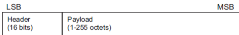
Figure 4: Advertising Channel PDU format. Source [2].
