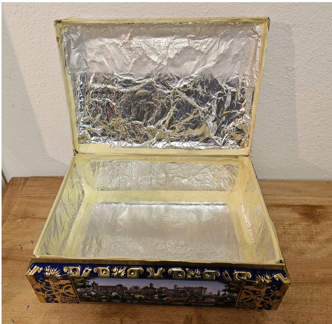
Figure 4.1: The Faraday Cage (metal Box)
