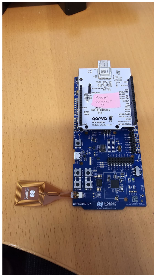
Figure 3.3: Combination of nRF52840 and DWM3000EVB
