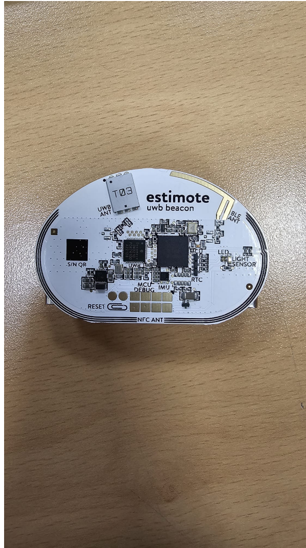
Figure 3.4: Inside of a UWB beacon designed and produced by Estimote Inc.
