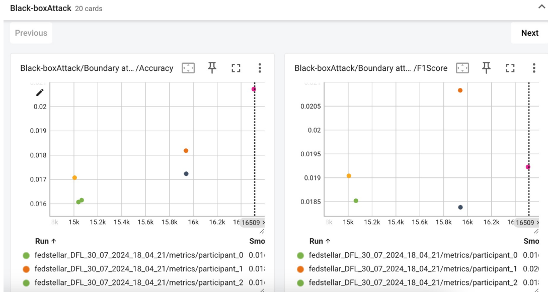
Figure 4.4: Black-box Attack Performance Logging in Fedstellar Tensorboard
