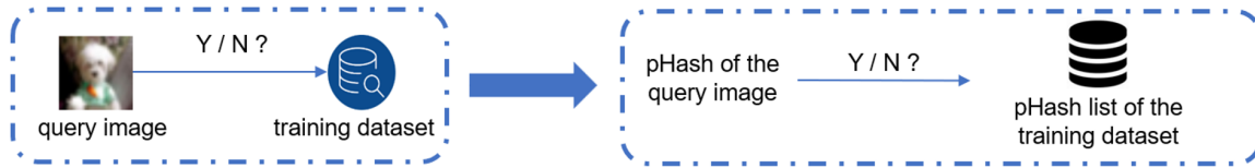
Figure 4.2: Determining Whether the Query Image is in the Training Dataset
