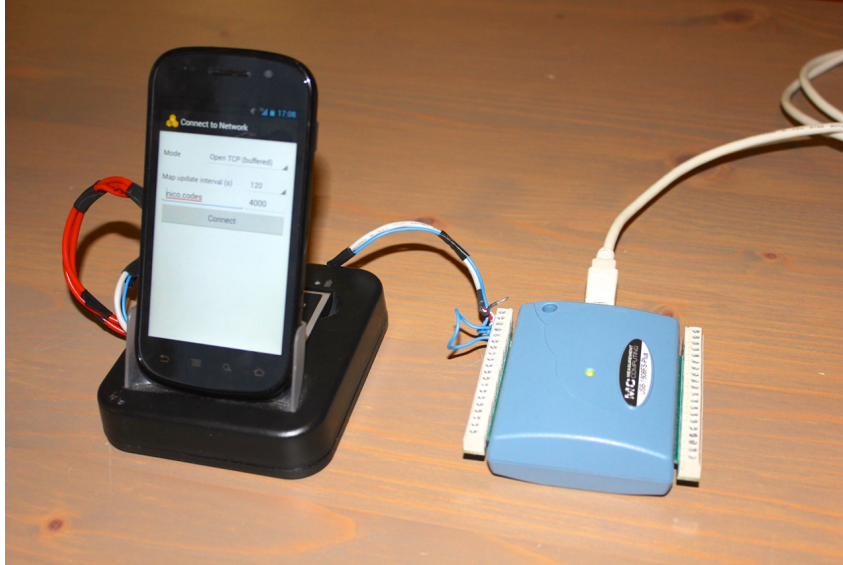
Figure 5.1: A data acquisition device is wired to a docking station to measure the energy consumption of the mobile phone.
