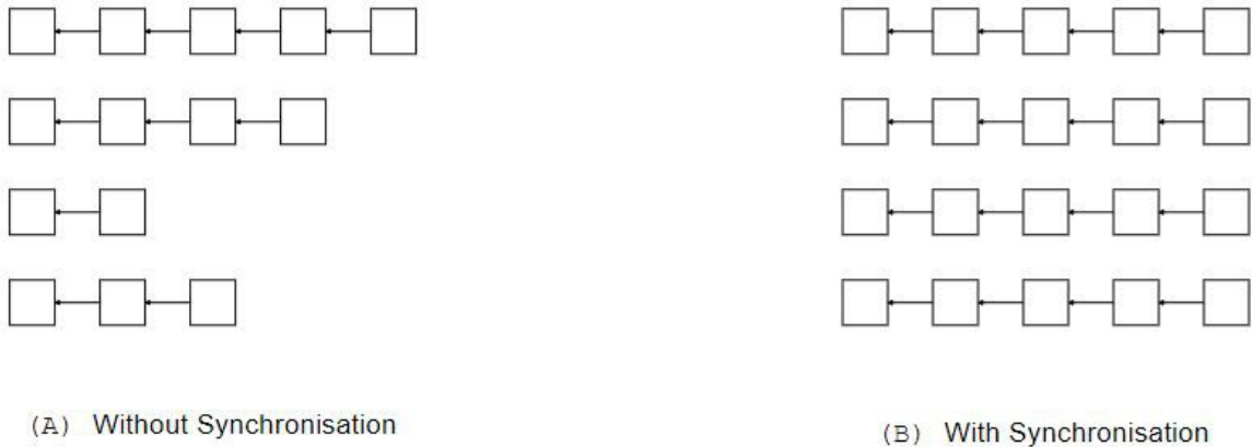
Figure 3.4: Due To Network Latency And The Speed Of The PoS, Shard Chains Might Diverge, Resulting In Different Block Heights
